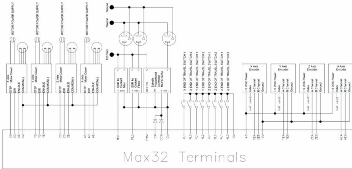
**Diagram 1 - Typical Motor Connection**
