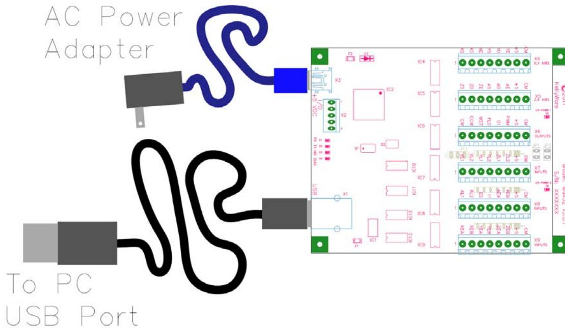
**Diagram 2 – PC USB Port and Power Supply Connection**
